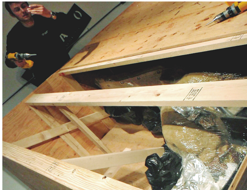
A shock-isolation system was designed to sustain the 4,000-lb specimen using foam padding on which the entire crate rode.
